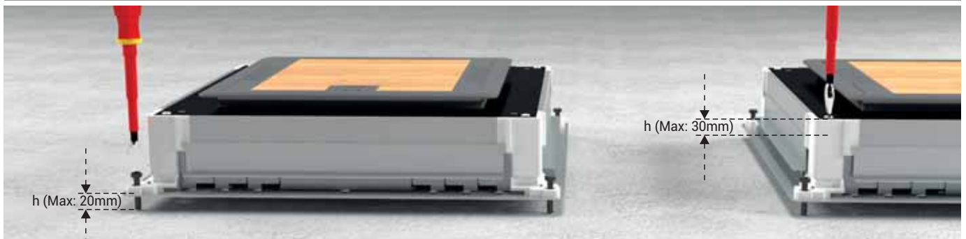
Before Screed Height Adjustment (20mm)
